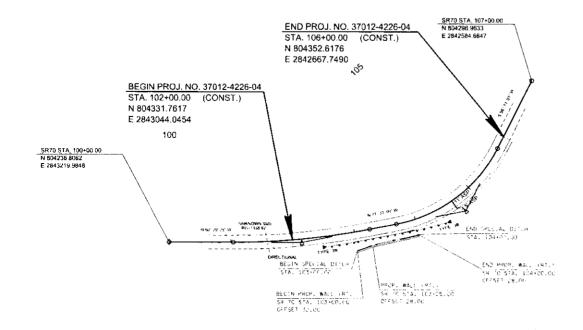
NOTE: SPECIAL DITCH WILL BE DESIGNED BY THE CONTRACTOR | 45 PART OF THE RETAINING WALL DESIGN
